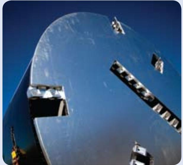
Weighing nearly 40 tonnes, the underground boring machine has a 2.8 metre rotating cutting face which can bore up to 12 metres per day, depending on ground conditions.
